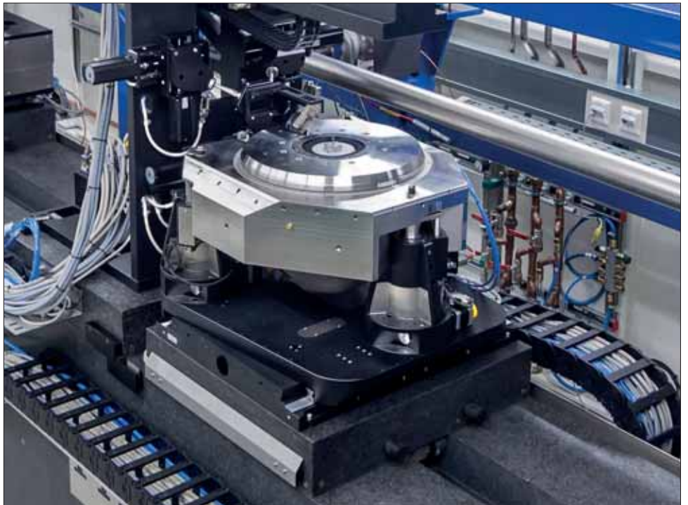
Mounted on the combined tilt and Z stage (consisting of three differentially controlled lifting elements) is an air-bearing supported rotation stage. It rotates at a velocity of up to 36°/s and works with flatness deviations of less than 100 nm at a resolution of 0.5 μrad (Image: PI / HZG)
