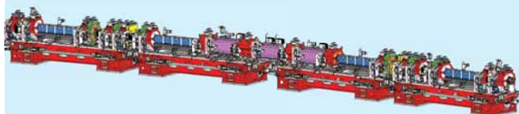
One cell of the EBS's HMBA lattice, supported on its four girders. There are four dipoles (blue) and three dipole-quadrupoles (pink), making seven bending magnets in total. Also shown are quadrupoles (red) and sextupoles (green).
